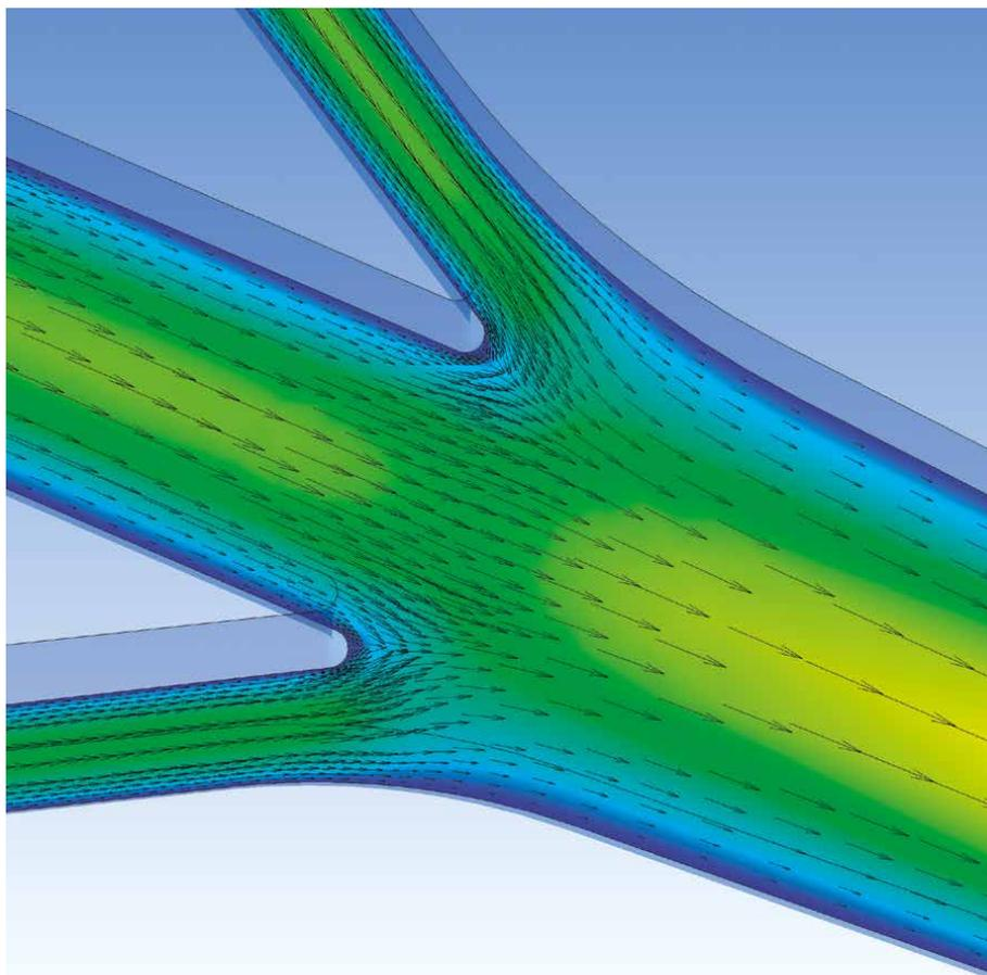
3D simulation for analyzing the material flow in the extrusion head
