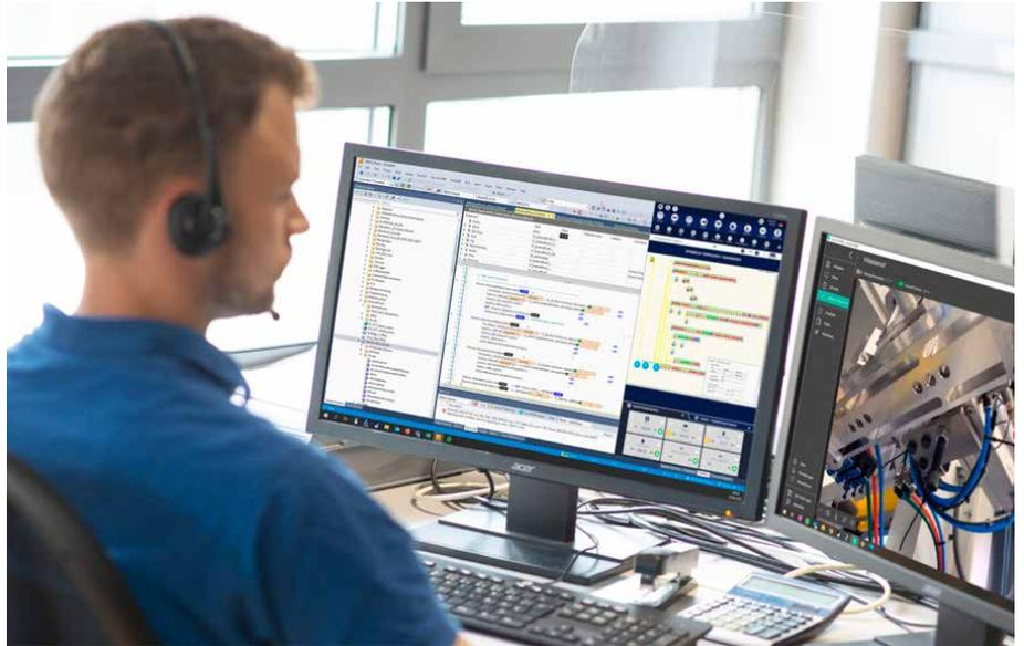
board of the ID 4.0-capable BC 8.0 machine control system, with the user being able to customize its layout. The operator has an overview of all consumption media "that my machine currently needs." Access to historic data is also configured.
