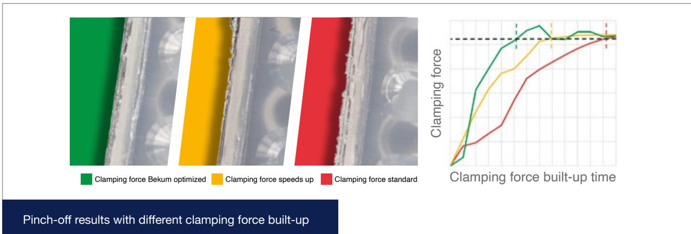
Pinch-off results with different clamping force built-up
