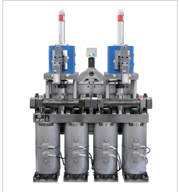
Spiral mandrel extrusion head for reproducible production qualities
