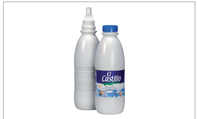
1,5 litre milk bottle made of 3-layer HDPE and recycled materials, blow moulded in a sterile process
