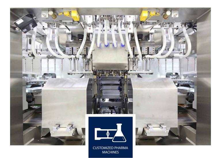
All-electric blow moulding machine for clean room operation
